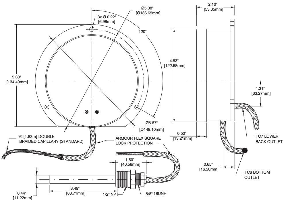
**REMOTE READING THERMOMETER MANUFACTURED AT OUR PLANT**
